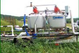
Cart mounted filter component of the microirrigation system
