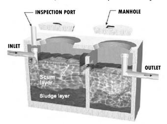
field. If the tank is not periodically pumped out, these solids will eventually clog the pipes and/or soil pores in the absorption (leach) field to the point where a new sand mound will be needed.
