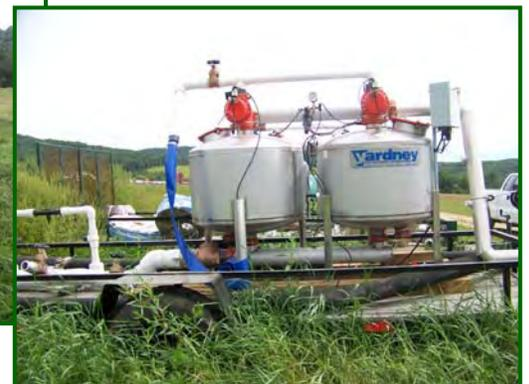
*Cart mounted filter component of the microirrigation system*
